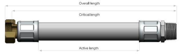
**Critical length** is the distance between hose mating faces. This must be 10% greater than the actual distance between the two corresponding fixed mating parts to avoid tensile stress whilst in service.
