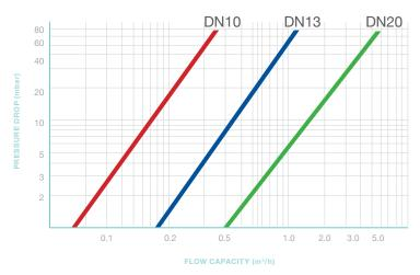
Therefore pressure drop (mbar) can be calculated for any given hose assembly adding P1 and P2
